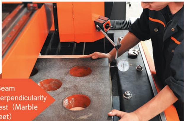
Beam perpendicularity test (Marble feet)
