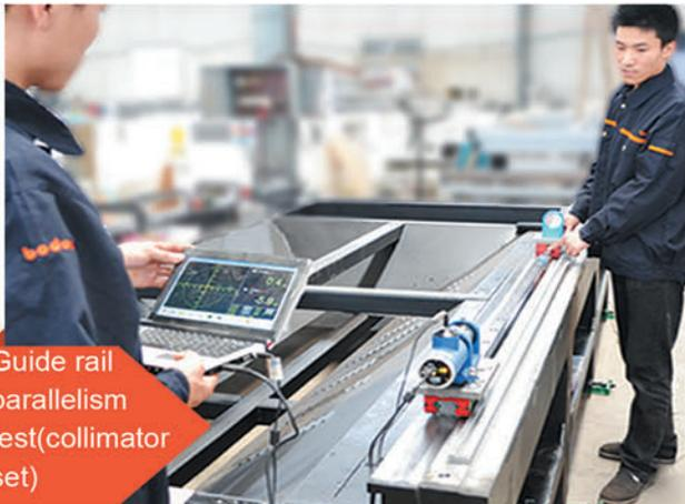
Guide rail parallelism test(collimator set)
