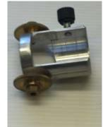
The circle cutting attachment is very easy to work with. Simply snap in the torch in the holder and adjust the centrepiece to the correct radius. The torch can rotate in its holder, which helps the operator to complete a full circle without having to stop and change grip.
