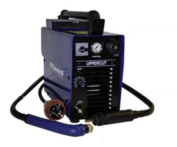
**UPPERCUT** is a 120A portable air-plasma system with extremely high performance in relation to its low weight, the power source weighs only 18 kg and can cut up to 45mm thickness. With air plasma systems you can cut mild steel, stainless steel, aluminum, brass, copper and other electrically conductive materials.
